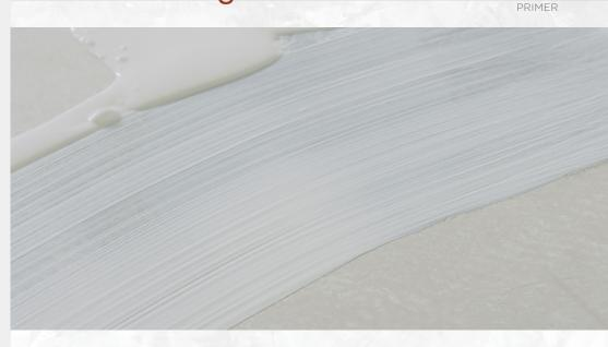
Siena Self-Leveling Primer is a latex based primer for use with Siena Self-Leveling Underlayment (SLU). It is solvent free and improves the underlayment's bond over porous substrates. Siena Self-Leveling Primer is a white liquid that dries clear. It is recommended that Siena Self-Leveling Primer be used in all self-leveling install projects.
